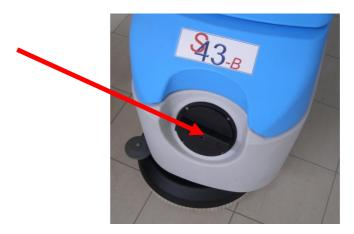
**WARNING**: before beginning the cleaning work, ensure that the brush fitted to the machine is suitable for the type of floor surface to be cleaned: too soft would not have much cleaning power, whereas too hard would damage the floor surface. Our technician/salesman can certainly be of assistance on this and any other matters.
